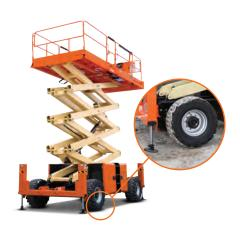
Foam-filled tires reduce the need for additional counterweight to meet new stability test standards.
