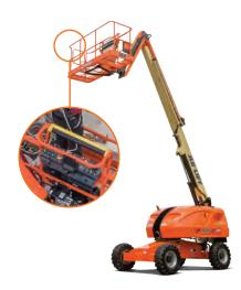
SkyGuard comes standard on most boom lifts. When activated, it sounds an audiovisual alarm and reverses most functions in use at the time.
